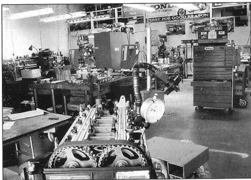
Working with overhead cam engines means the max lift occurs when the valve travels farthest away from the dial indicator.
